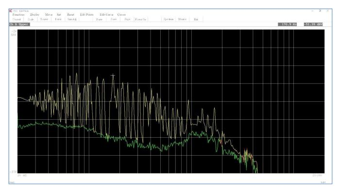
P900 test is used with a TRK-HP filter in channel B. The test sweep is from 20 to 20 KHZ. If the test is repeated the behaver will be different from this example.
