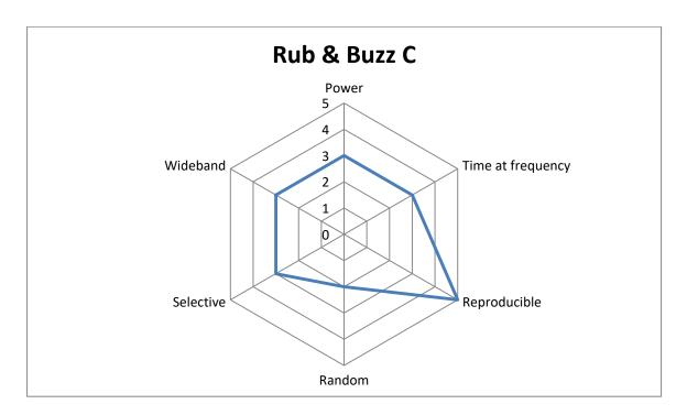
D) Buzzing signal as selective resonance generated due to some missing gluing.
