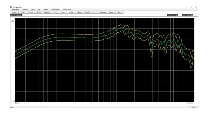
In the following example only frequency curve limits are used. The limits are moved  $\pm$ -2 db. Here are used 10 good units. The difference from only use 1 unit and now using 10 units see in this case at frequency higher than 4000 Hz.
