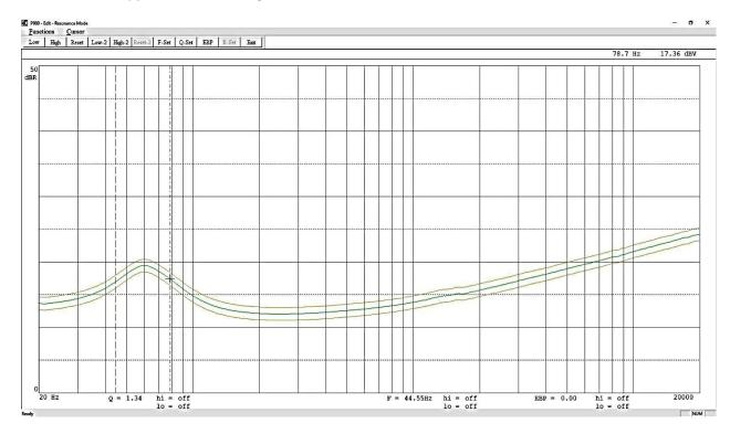
Test envelope for Frequency response is used +/- 3 db. In this case the sensitivity has to be within this envelope.
