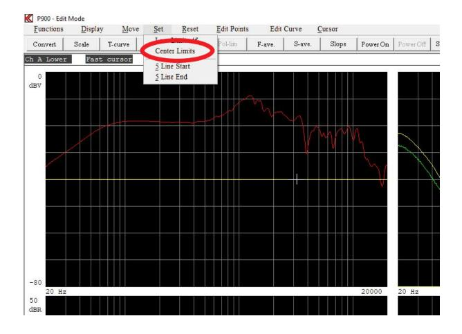
The Frequency Jitter widen can used if there is a resonance and this make is difficult to edit reference points. The Jitter moves the reference points +/- 1 frequency points every this function are called. The function is called from the "Move menu"
