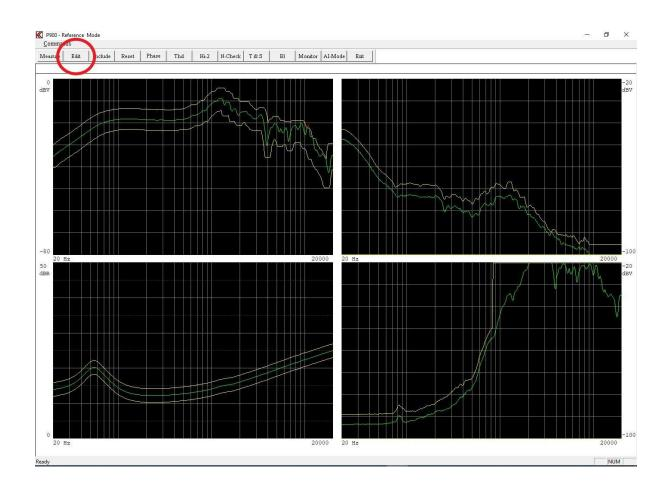
When enter the Edit Mode a cross cursor is seen on the Upper Reference as default. On the right readout of the cursor point is displayed with frequency and value.
