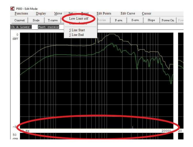
The upper and lower limits can be reset to the middle of a channel range at -40 db below of screen top (normally this is middle of the screen.
